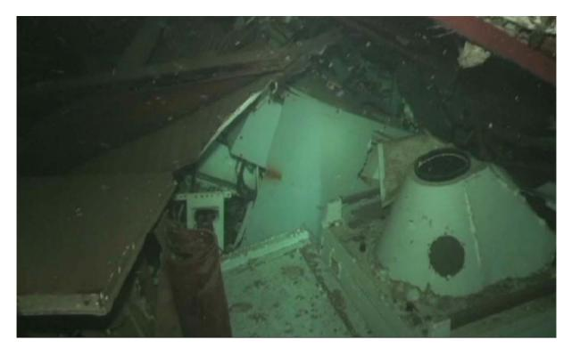
The navigation bridge is heavy bended down in the middle. Starboard side wing door of the bridge is opened and the port side wing one is closed.
