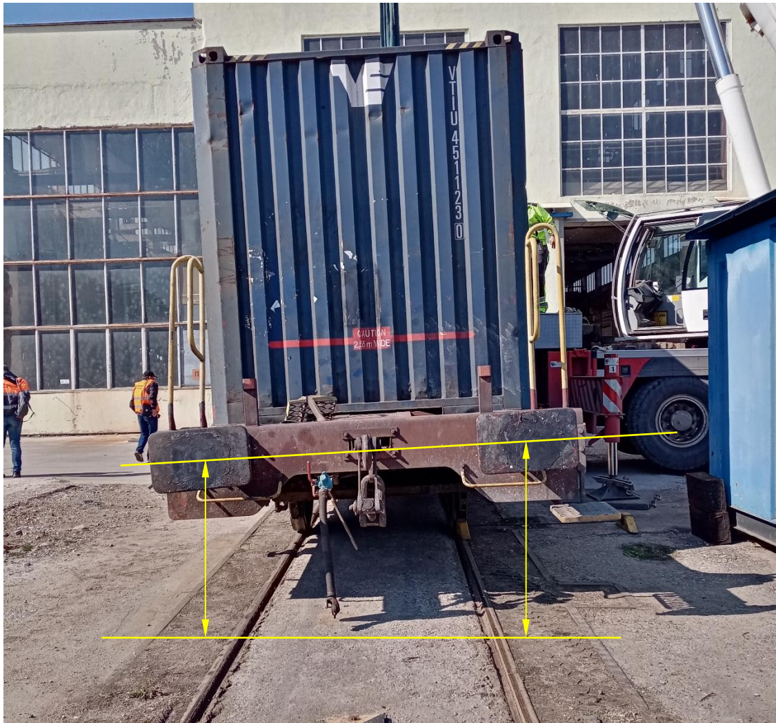
Fig. 4.16. On the image is shown the difference in height of the two buffers.
