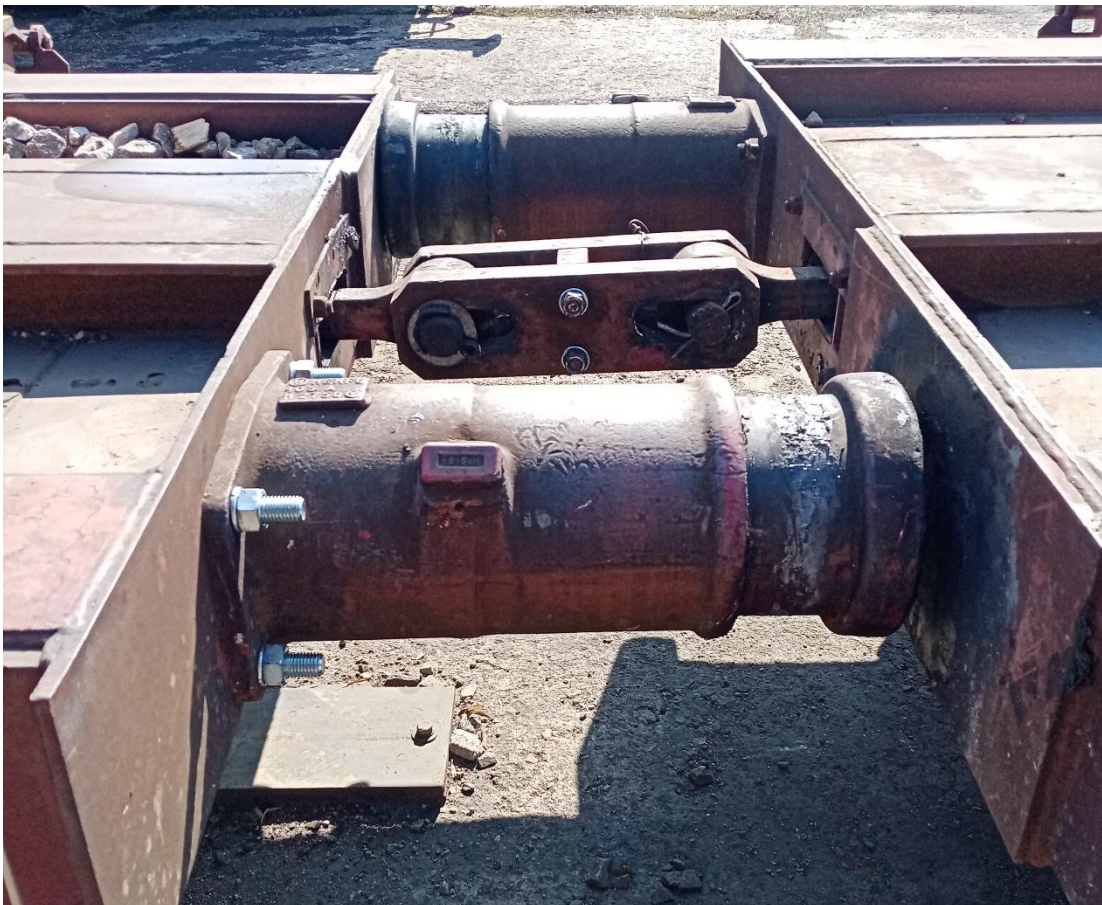
Fig. 4.12. Appearance of the device connecting the two platforms of wagon № 43714378583-4.
