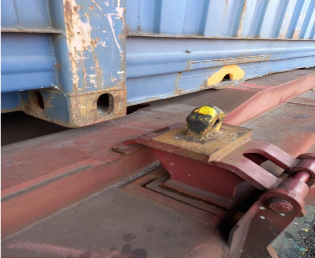
Fig. 4.13. Displaced container from the heel of the wagon.
