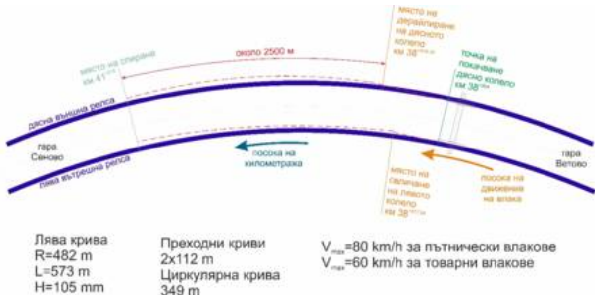
Fig. 4.14. Scheme of the derailment mechanism
