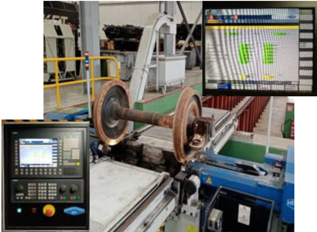
Fig. 4.7. Photo from the wheel-set measurement on the wheel-set lathe with the control board and the display with the results.
