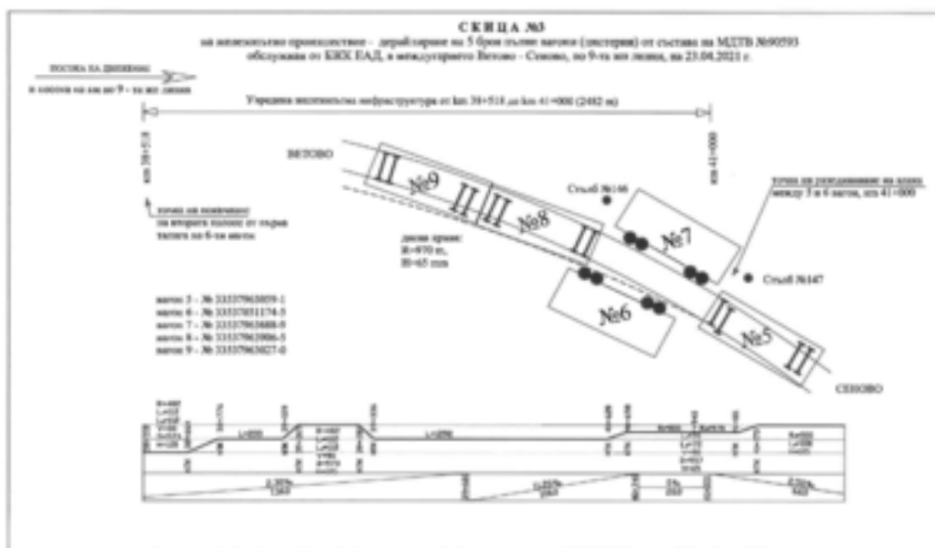
Fig. 1.6. Scheme № 3 – place of derailment of five wagons from the composition of DFT № 90593
