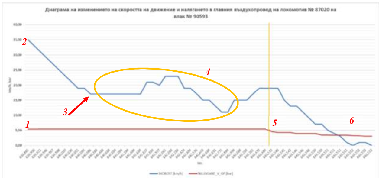
Fig. 4.5. Chart of the movement of DFT № 90593 of the registering device of locomotive № 91520087020-1 latest data before the derailment
