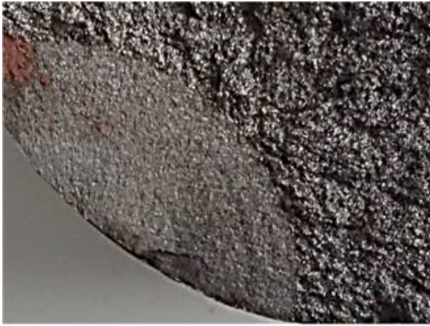
Fig.55. Fatigue grooves in zone A (OM)
