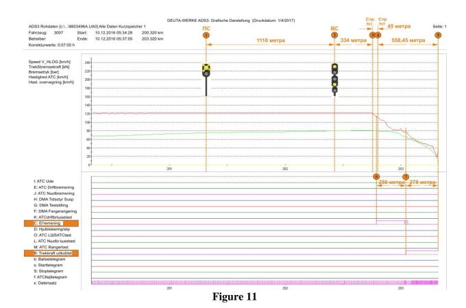
schedule it reached 81 km/h (marker ③ on Figure 11). At the warning traffic lights (marker ①) the train passed with the speed of 78 km/h, and at the entrance traffic lights (marker ②) – with 80 km/h.
