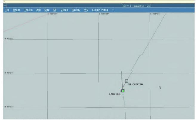
17:20:20 on 07.03.2013 m/v,,Lady Gul" - Bearing to m/v,,St. Catrien" =  $20^\circ$ ; D = 3 cables. m/v,,St. Catrien" - Bearing to m/v,,Lady Gul" =  $200^\circ$ ; D = 3 cables. VTMIS – Varna
