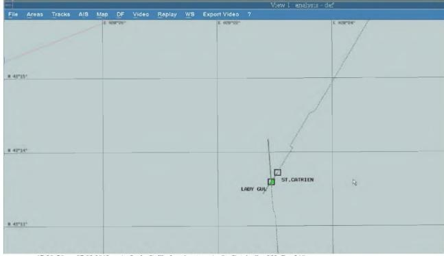
17:20:56 on 07.03.2013 m/v,,Lady Gul" - bearing to m/v,,St. Catrien" = 33 $^{\circ}$ ; D = 210 m. m/v,,St. Catrien" - bearing to m/v ,,Lady Gul" = 213 $^{\circ}$ ; D = 210 m. VTMIS – Varna
