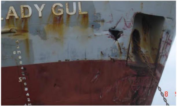
M/v"Lady Gul" – the hole after the collision on 07.03.2013 berth No. 1 - Varna.
