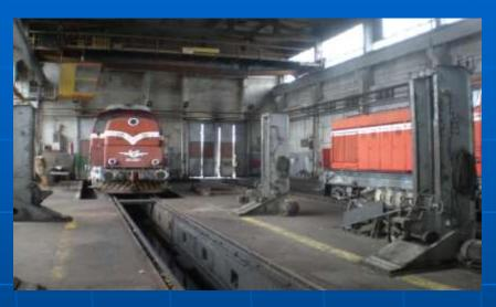
Engine yard – with facilities for maintenance and repairs of 1520 and 1435 gauge railway engines.
