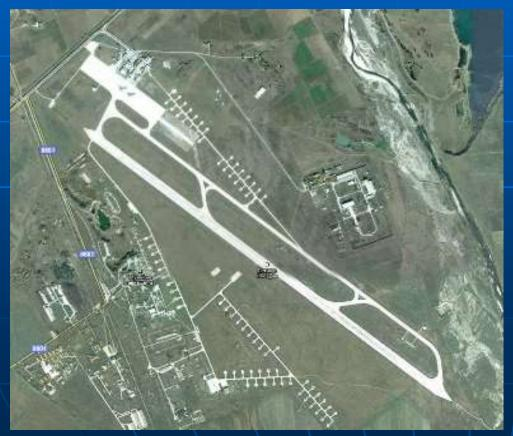
The size of the apron is 800 by 111 m. Most of the apron, 85 %, has concrete pavement, and 15 % are paved with asphalt. The apron has 13 aircraft berths, of which 6 are designed for type "C" aircraft, and 7 for type "D" aircraft. The apron pavement is in a good condition. The airport is equipped with instrument landing system (ILS) for Runway 30; landing at Runway 12 is subject to visual flights rules. The system used is D-3.
