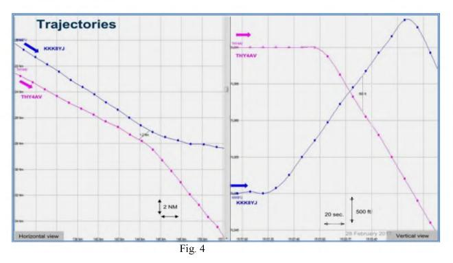
According to the simulation performed (Annex 2), the closest point of approximation occurred at 15:03:33 h. The horizontal distance between both the aircraft was 1.24 NM and the vertical was 500 ft. (See Fig. 4)
