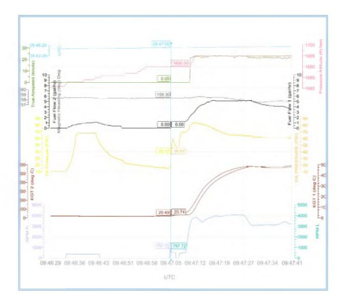
UTC 9:47:06 EGT 1: 23 deg C EGT 2: 27 deg C RPM L: 523 RPM R 523 Fuel Flow 1, 2: 0.7 gal/hr OIL PRESS: 58.5 PSI During the engine start the parameter Oil Press doesn't change.
