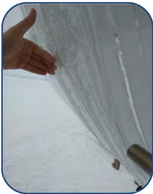
Zoom on Ice accretion on lower fuselage
