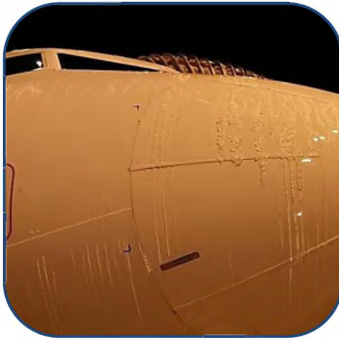
Zoom on Ice accretion on lower fuselage
