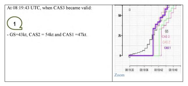
During take-off roll, CAS1 and CAS2 became valid first (i.e. increased above 30kt) then the CAS3 became valid 4s later meaning that CAS3 was not consistent with CAS1 and CAS2. When CAS3 reached 30 kt, the following airspeed discrepancies were recorded:
