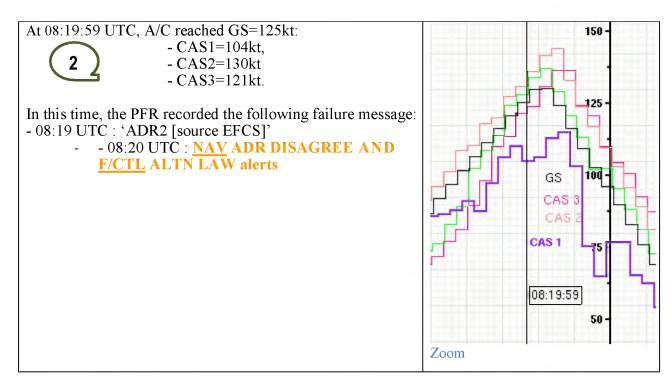
The message on ECAM and maintenance messages, the message NAV ADR DISAGREE was triggered most probably because ADR2 was already rejected by ELAC and whether another discrepancy was detected between the 2 remaining ADRs. As a result of at least two ADR rejected by EFCS, Flight control reverted to ALTERNATE LAW.
