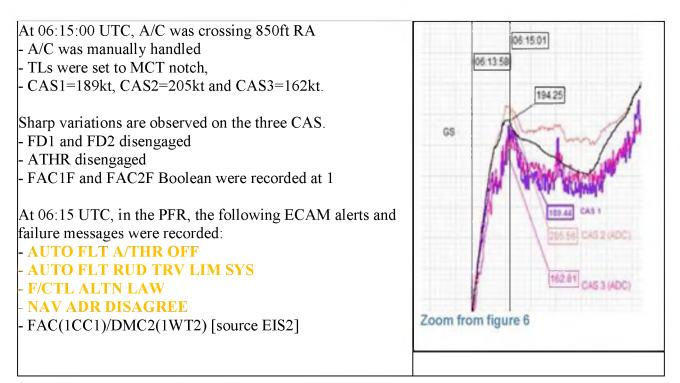
Then, during lift off, the CAS discrepancy has increased with a difference of more than 40kt between CAS1 and CAS3 (considering ADR2 already rejected).
